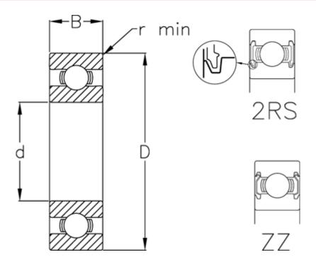
B = 16 d = 30 D = 62 Dynamic load C (kN) = 19.5 Max rpm greased = 11000 Max rpm oil lubricated = 13000
